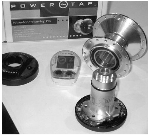
Figure 4.7 PowerTap measuring instrument. (Copyright Graber Products, 2001.)
