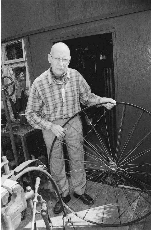
Figure 1.9 Starley-Hillman lever-tension wheel (circa 1870), shown by the late John Pinkerton in 2001. (Photo by Dave Wilson.)
